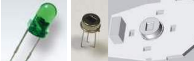
Sunlight Sensor Detects changes in Sunlight Intensity
